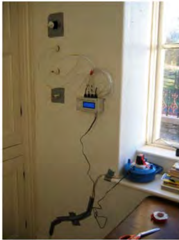
Figure 26. Interstitial monitoring set up at White House Farm, Skipton, 2011.
